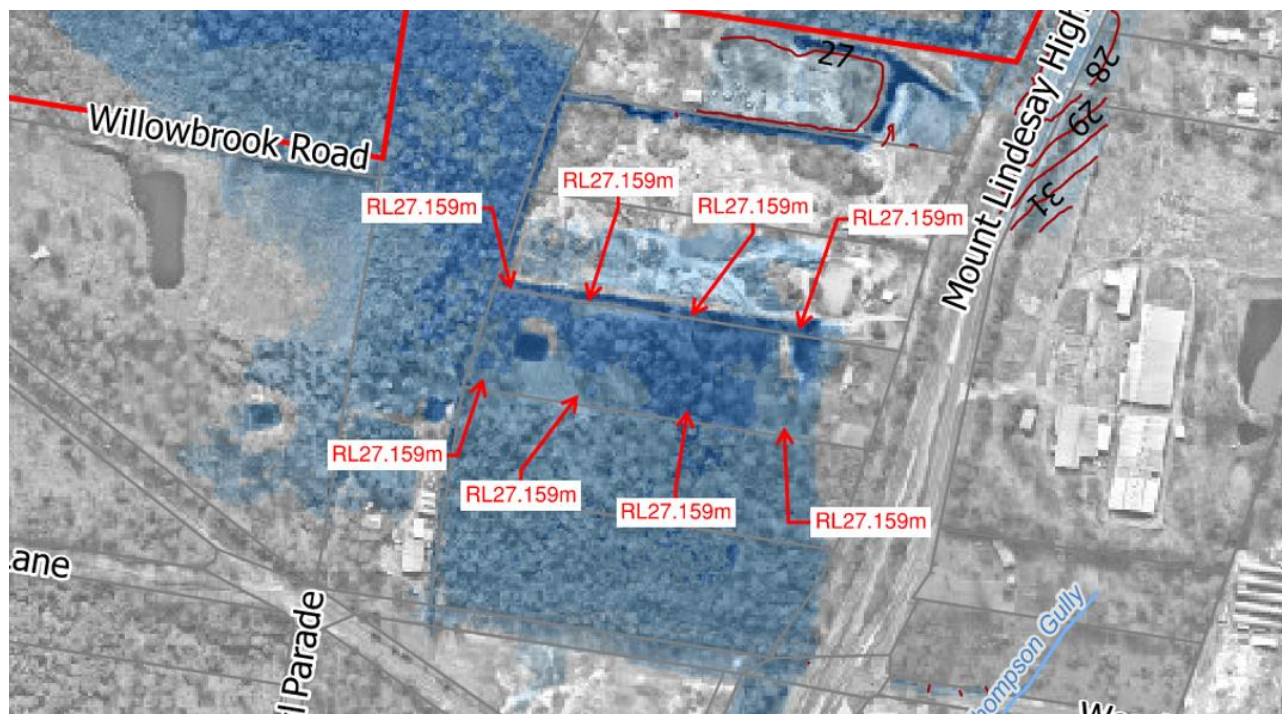
Figure 6.2 Flood Level Extracts for the Subject Site
