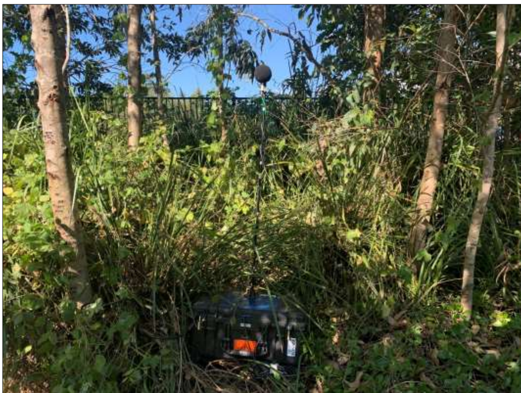
Photo: Logger Location 2 – Background Noise Measurements
