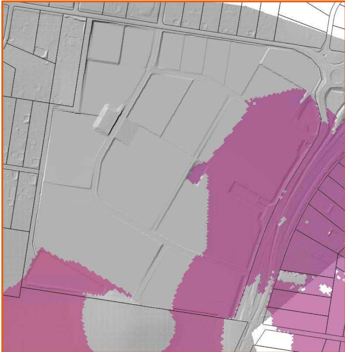
Figure 7 – Base Case 0.2% AEP (500 year) at 2100 flood inundation.
