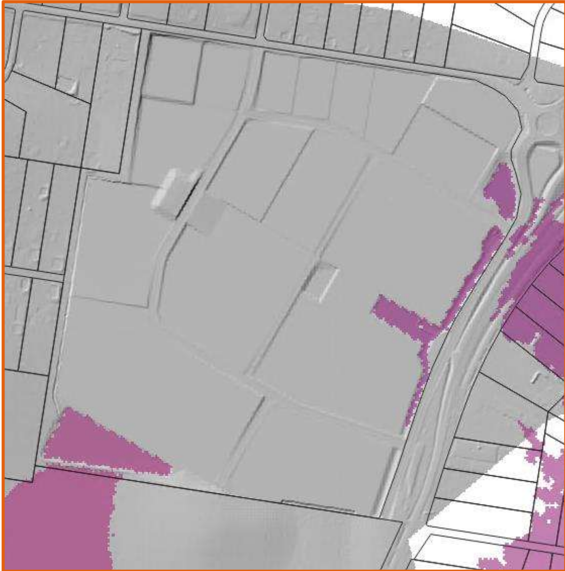
Figure 6 – Base Case 1.0% AEP (100 year) at 2100 flood inundation.
