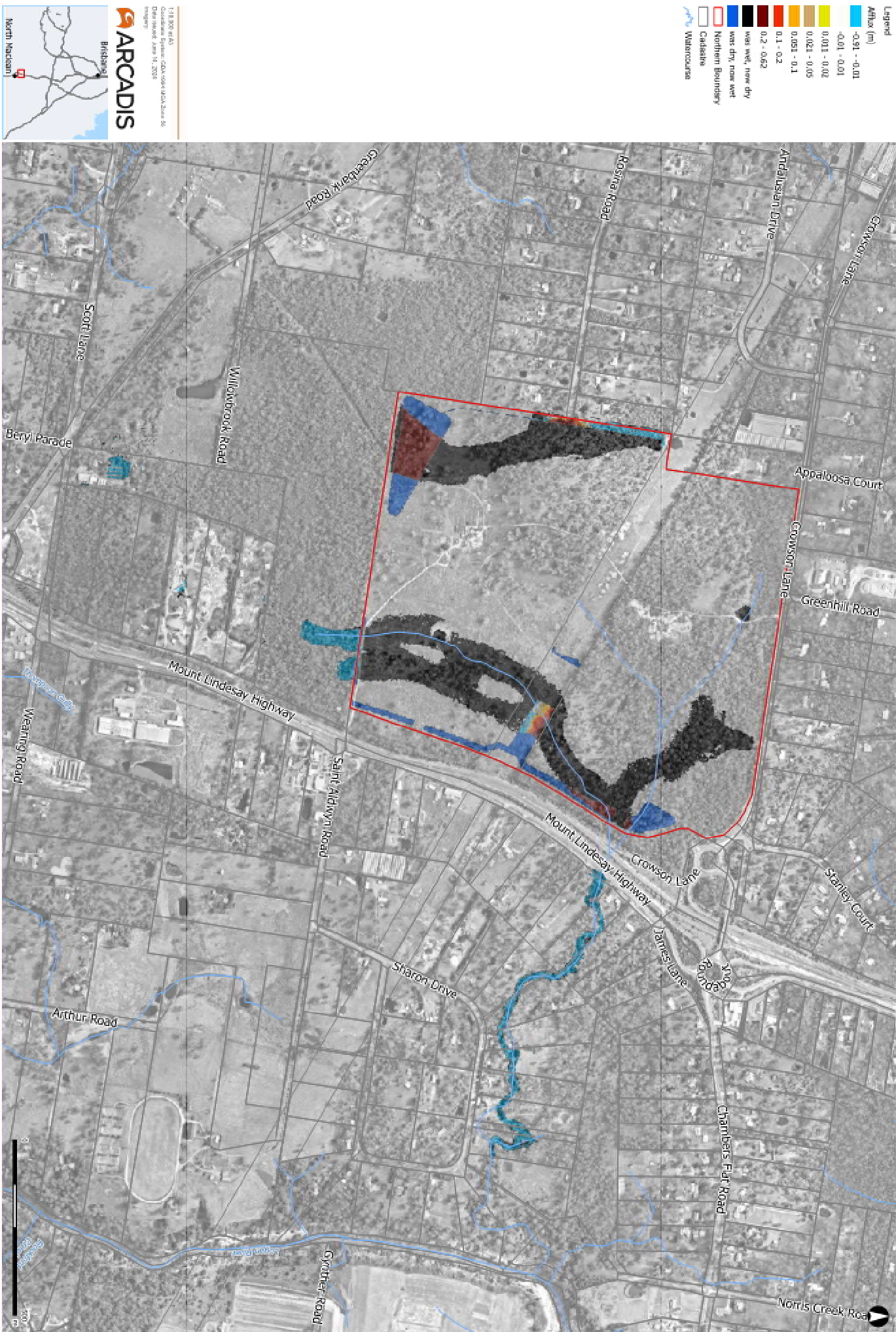
Figure D-16 - Flood Level Afflux - 5% AEP
