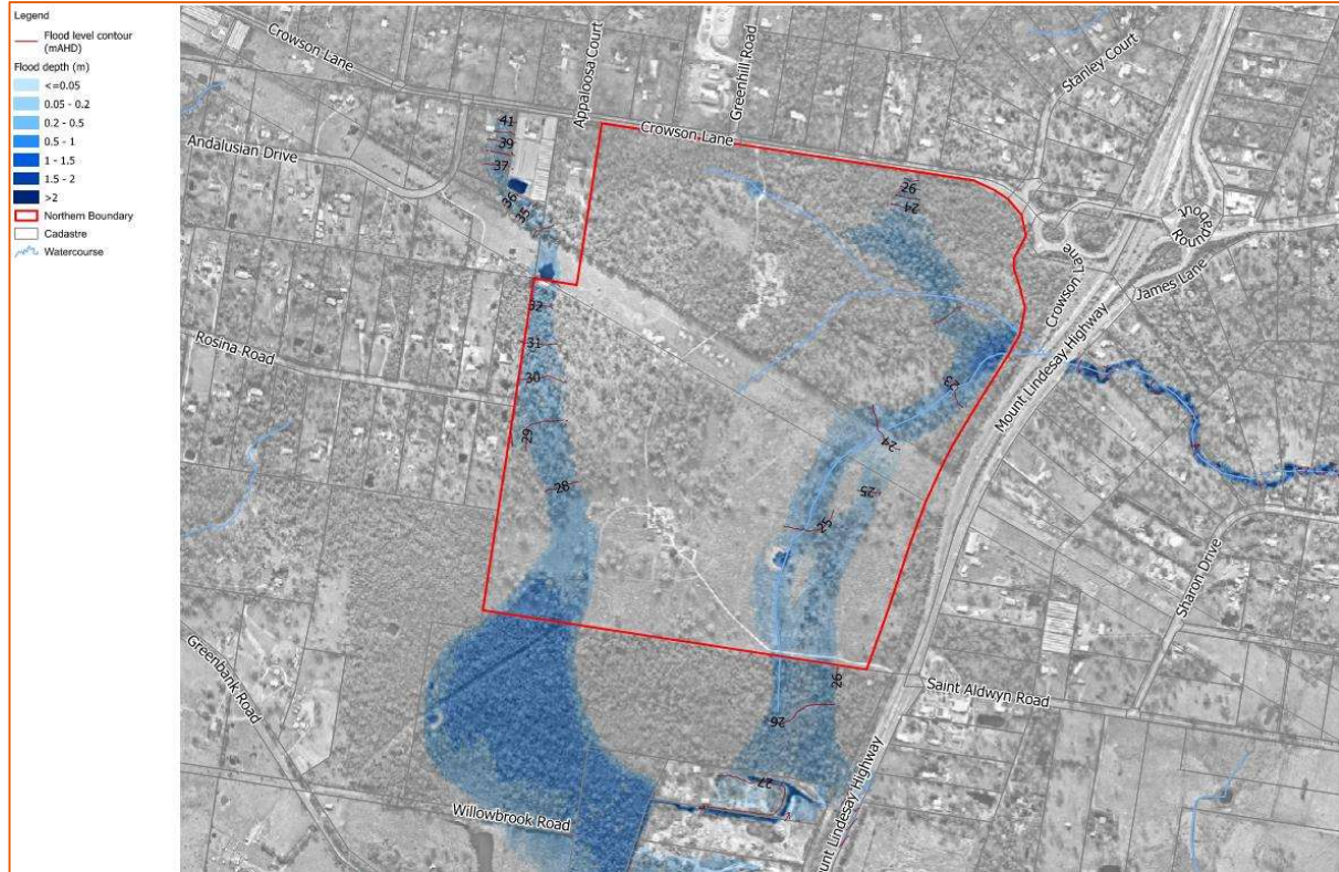
Figure 6-1 - Existing Peak Water Depth - 1% AEP
