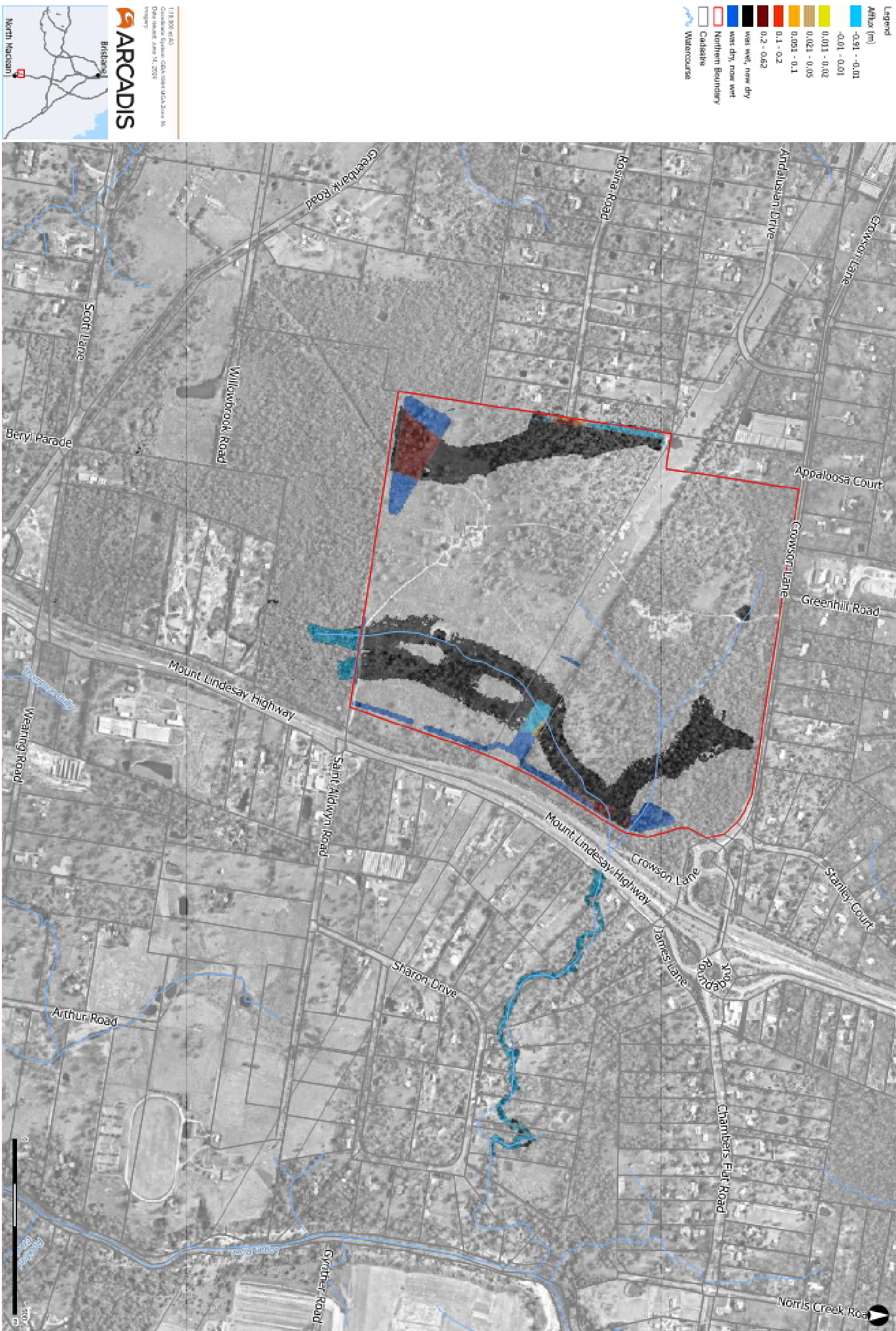
Figure D-15 - Flood Level Afflux - 10% AEP
