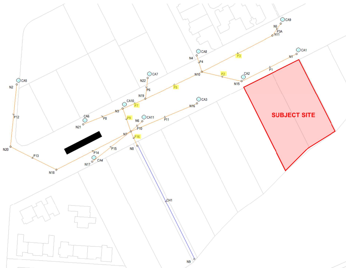
Figure 5-3: DRAINS Model Layout – Fully Developed Catchment
