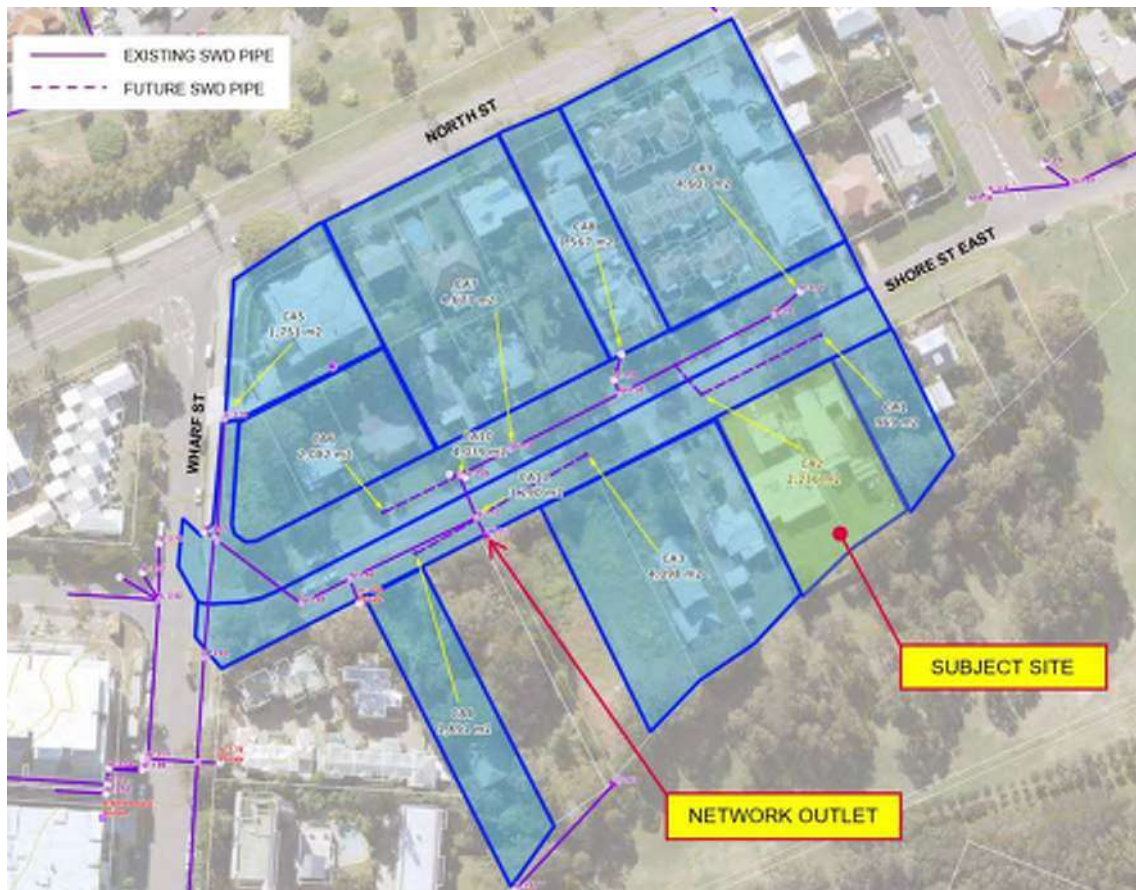
Figure 5-2: Fully Developed Catchments – Shore St East Drainage Network
