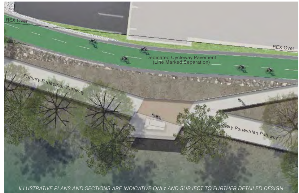
Figure 5.46: Goodwill Extension Type 1 Typical Pavement Treatment
