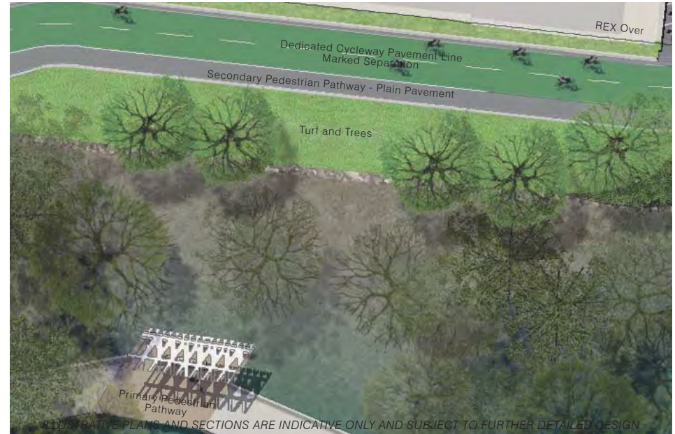
Figure 5.50: Goodwill Extension Type 3 Typical Pavement Treatment
