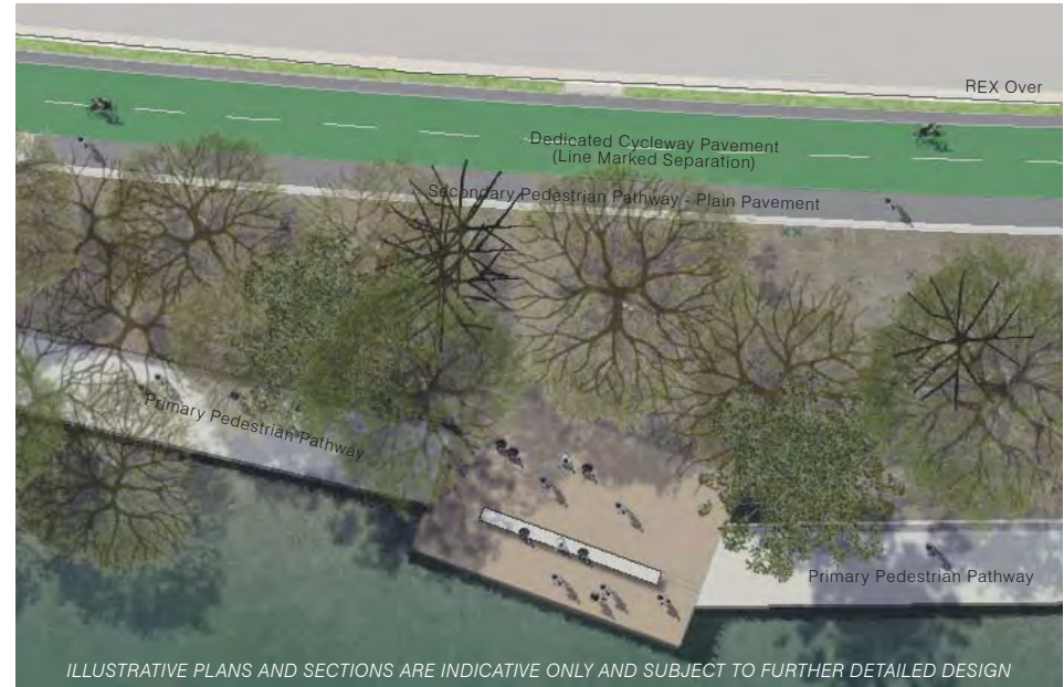
Figure 5.48: Goodwill Extension Type 2 Typical Pavement Treatment
