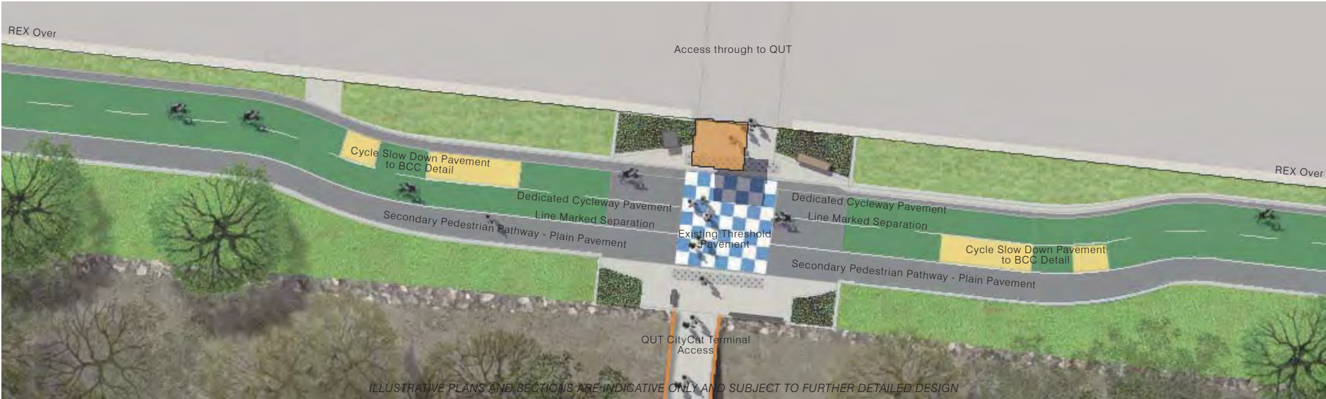
Figure 5.57: Transition Zone E Typical Pavement Treatment
