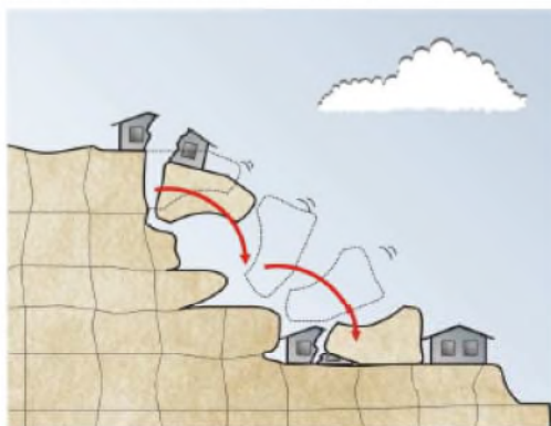
Figure 1 - Failure of an undercut block
