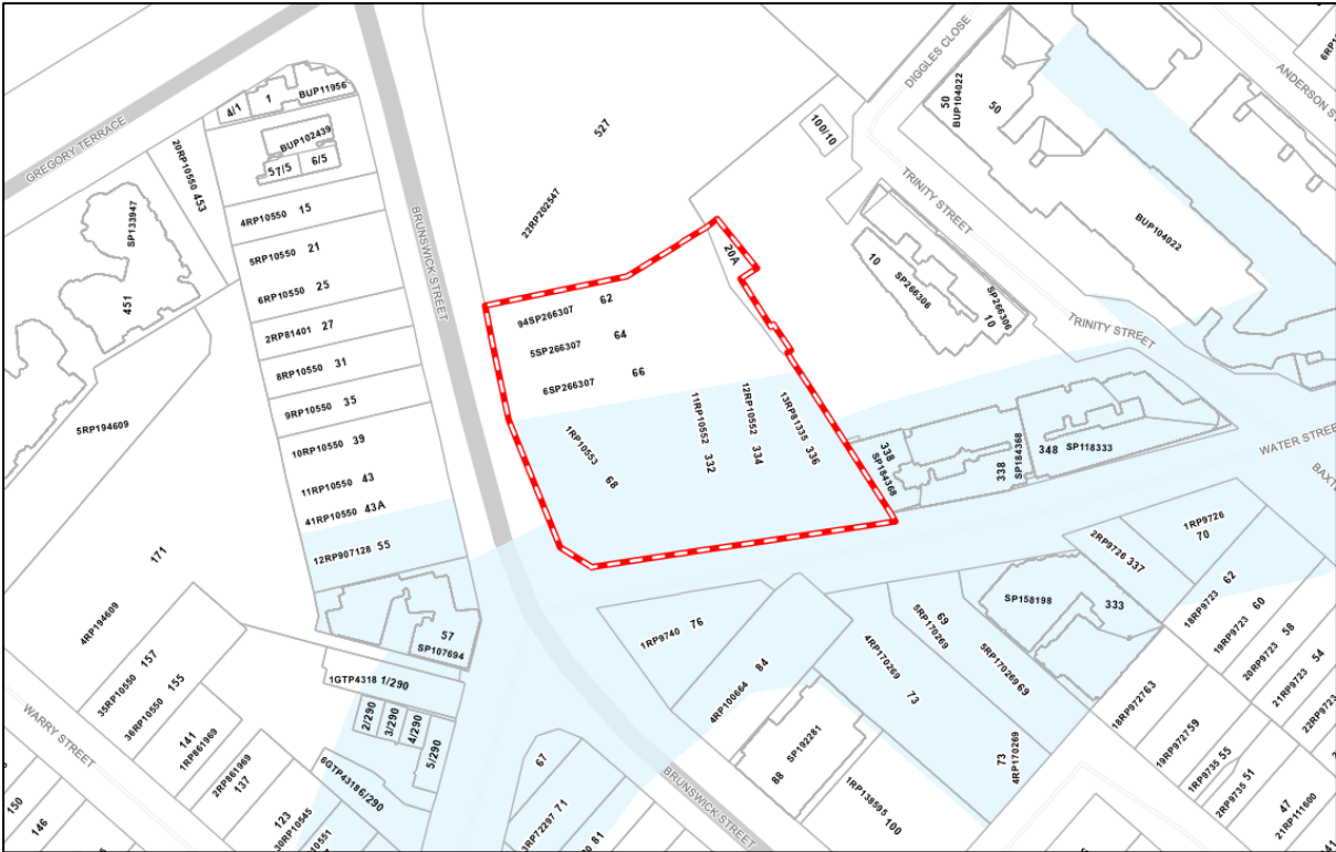
Figure 17 - Overland Flow Path
