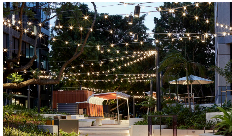
Overhead lighting on tensile structures using building columns to help define space or draw pedestrians into site
