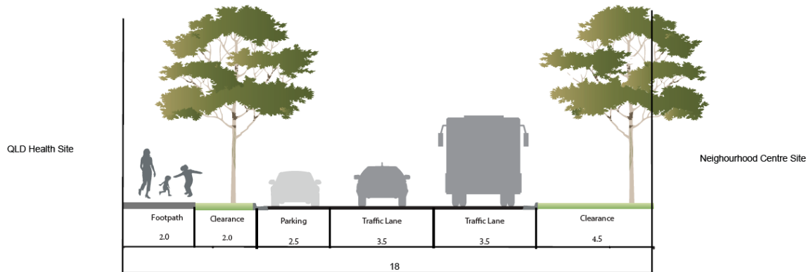
Access Street Section A - Cross-Section
