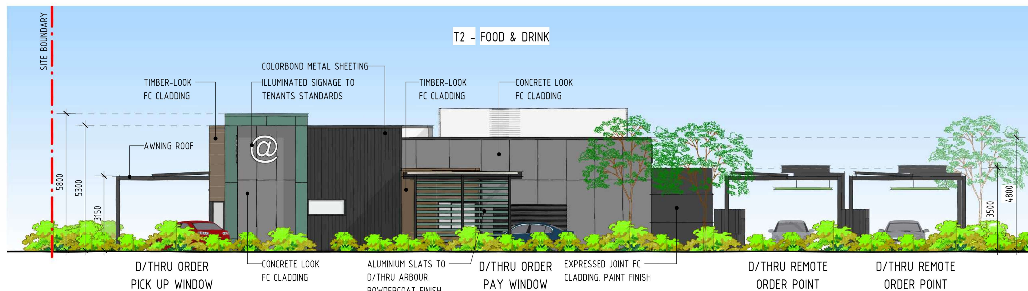
4 T2 - PROP. NORTH ELEVATION 1 : 100
