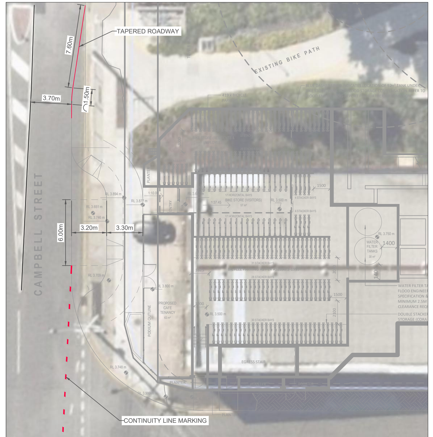
PASSENGER LOADING ZONE IN ACCORDANCE WITH BCC STANDARD DRAWING BSD-3162 INSET B 1:200
