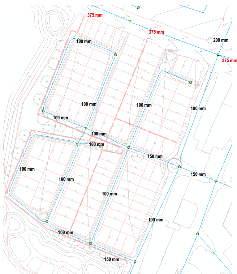
Figure 3 Water Reticulation Network for Precinct 4G
