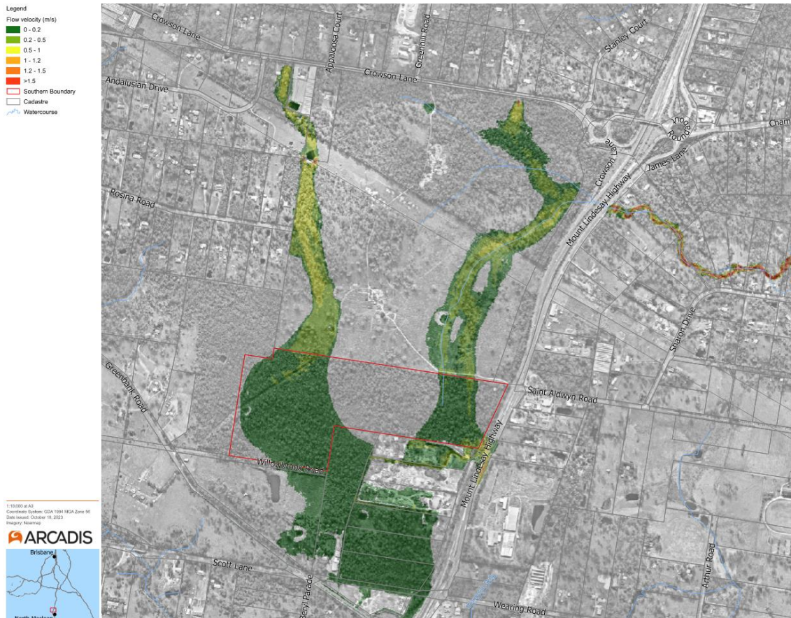
Figure 6-4 - Existing Peak Water Velocity - 1% AEP
