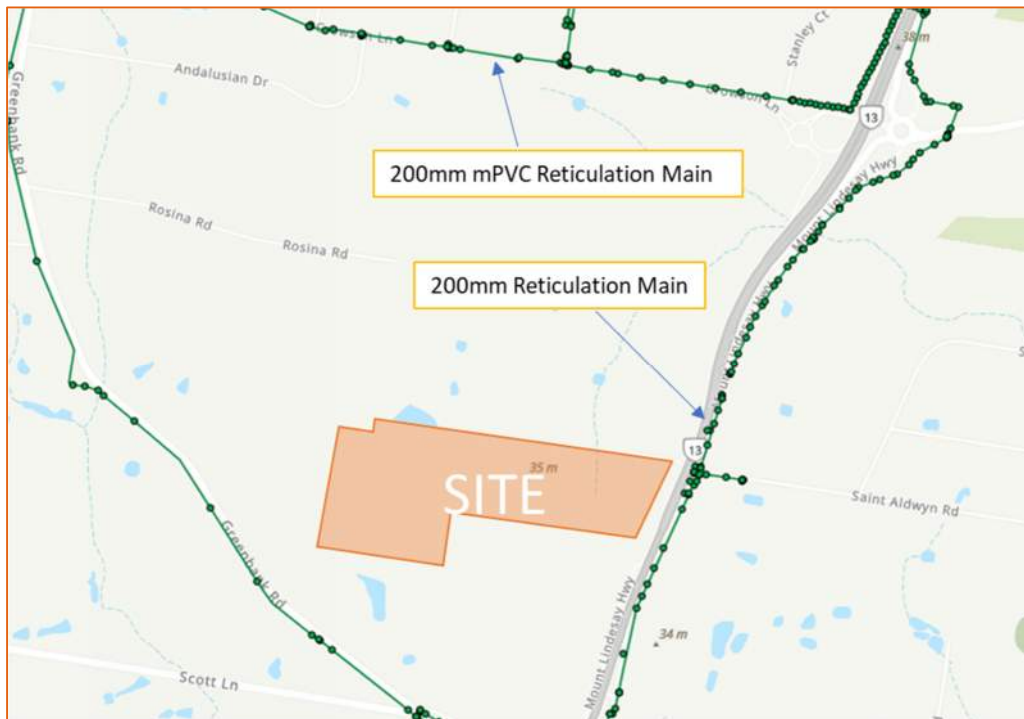
Figure 5-1 – Existing Potable Water Infrastructure
