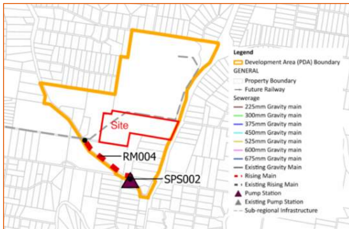
Figure 4-3 – Sewer Trunk Infrastructure in DCOP
