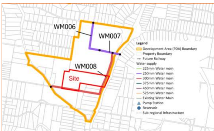
Figure 4-2 – Water Supply Trunk Infrastructure in DCOP
