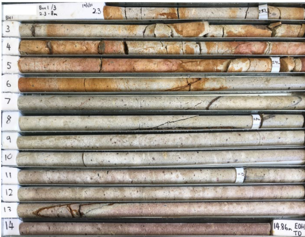
Image 11 – Rock Core sample in Tuff
