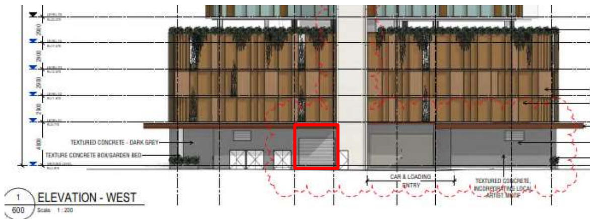
Figure 2 – Generator plantroom Western elevation
