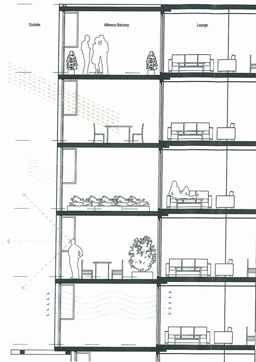
2 Alfresco Balcony Section - Facing North SCALE 1:50 @ A1
