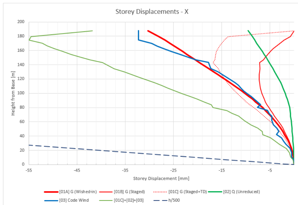
Figure 3: Building Lateral Displacements in X Direction (E-W)
