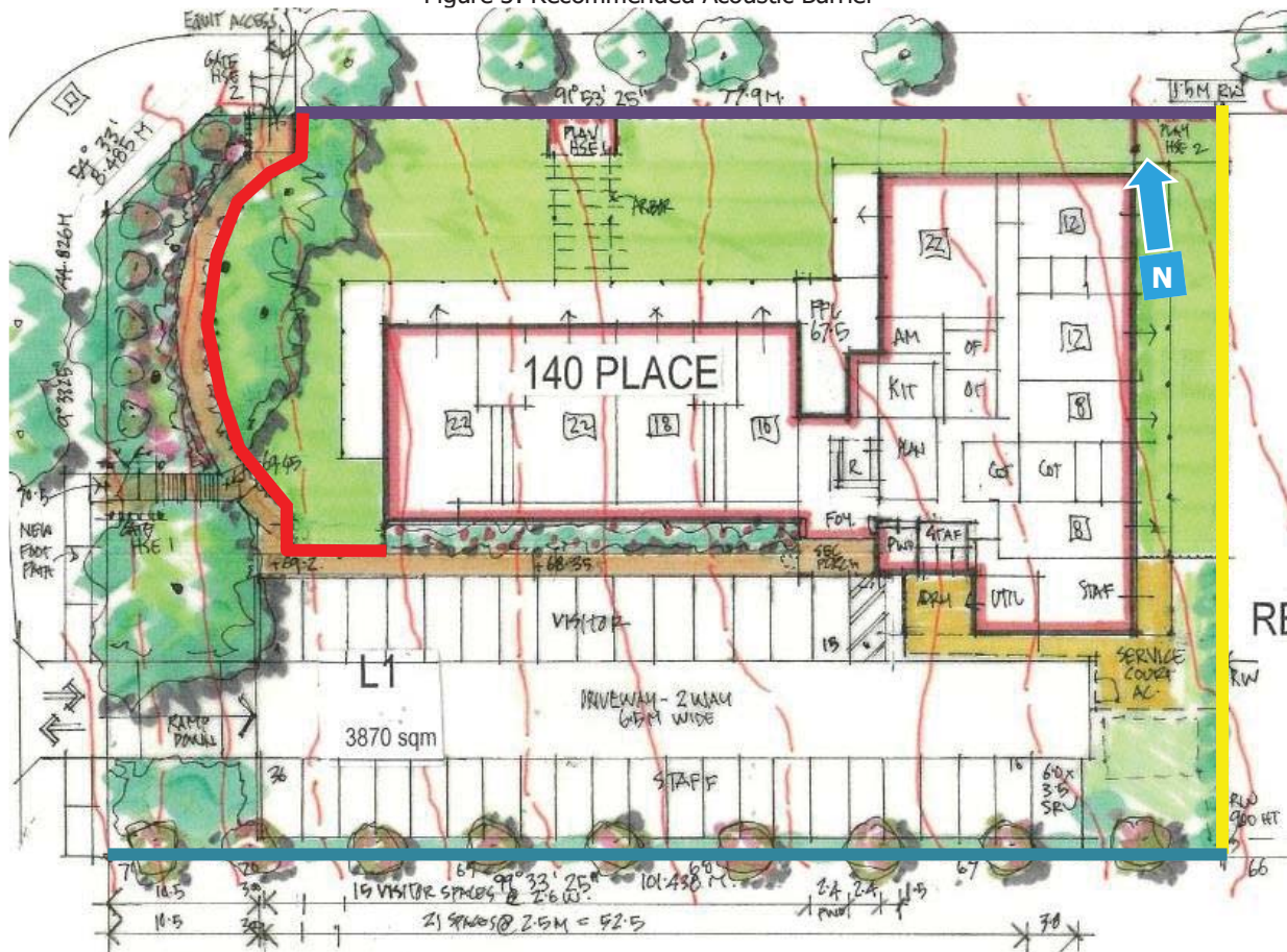
Figure 3: Recommended Acoustic Barrier
