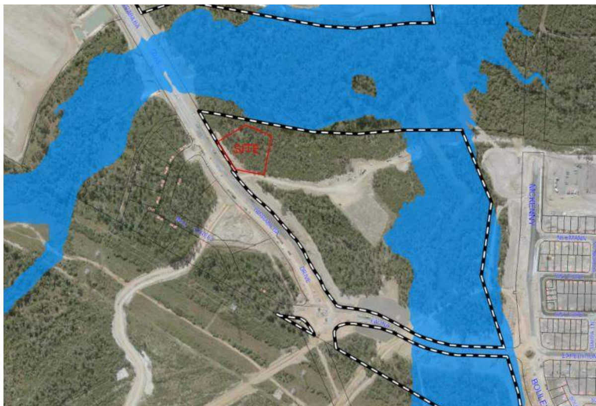
Figure 7.1 – Extents of Flooding (1% AEP Event)
