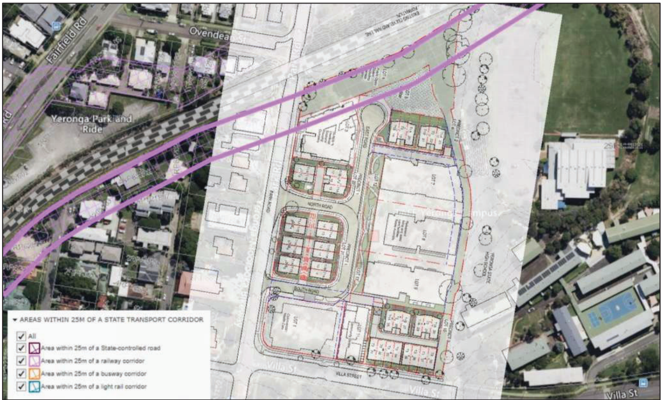
Figure 4: Areas within 25m of State transport corridor
