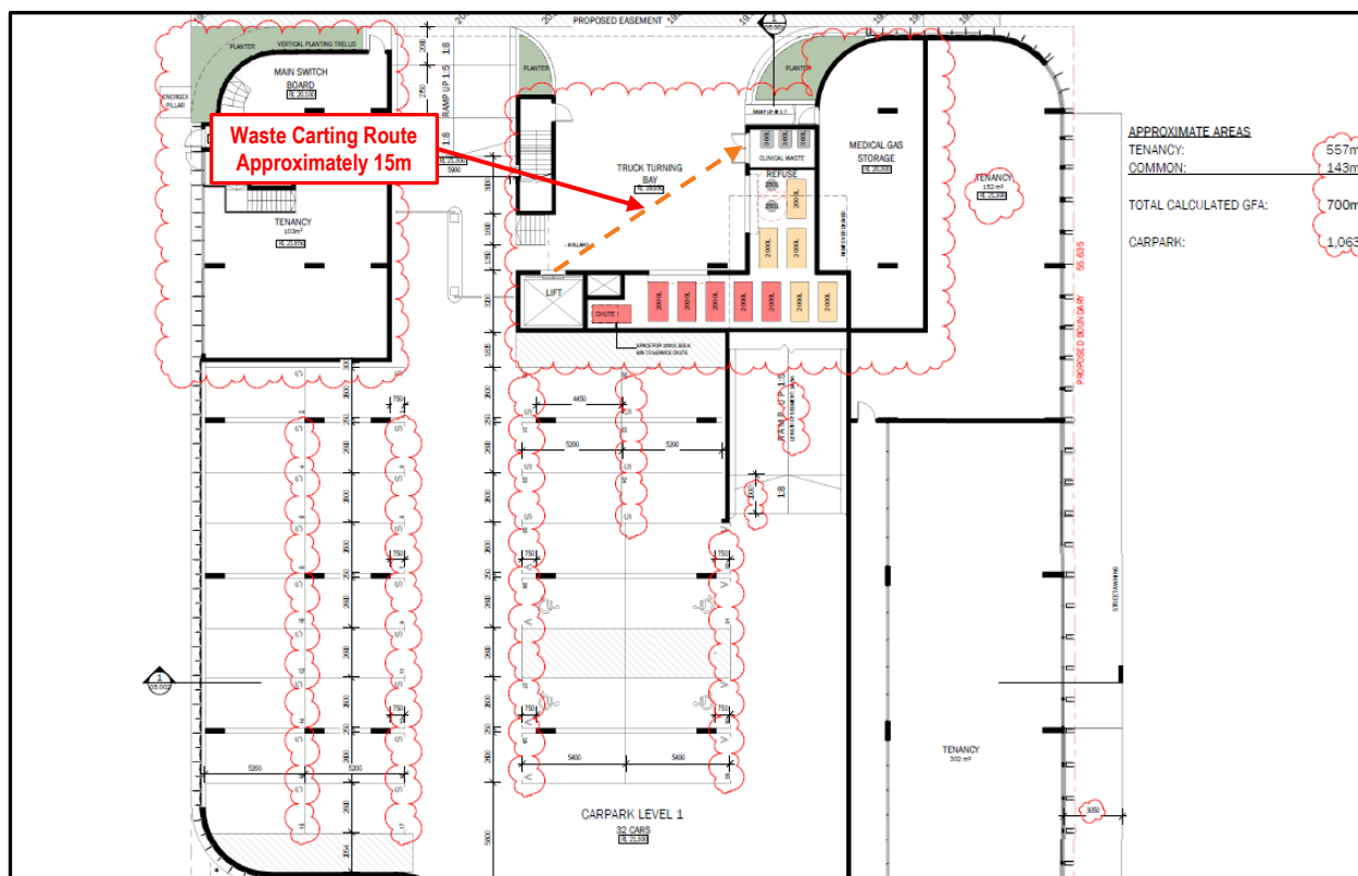
Figure 3.5.5 Typical Waste Carting Route (Level 1 Shown)
