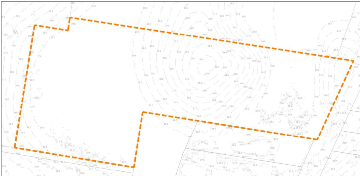
Figure 3-4 - Existing Site Contours (LiDAR)
