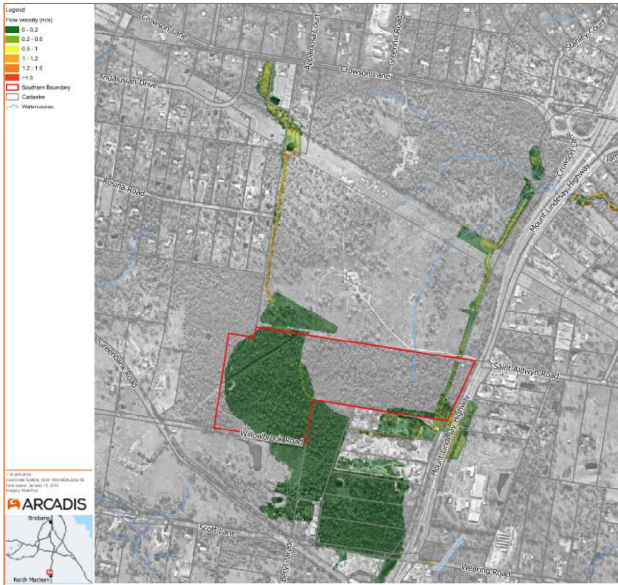
Figure 6-5 - Developed Peak Water Velocity - 1% AEP
