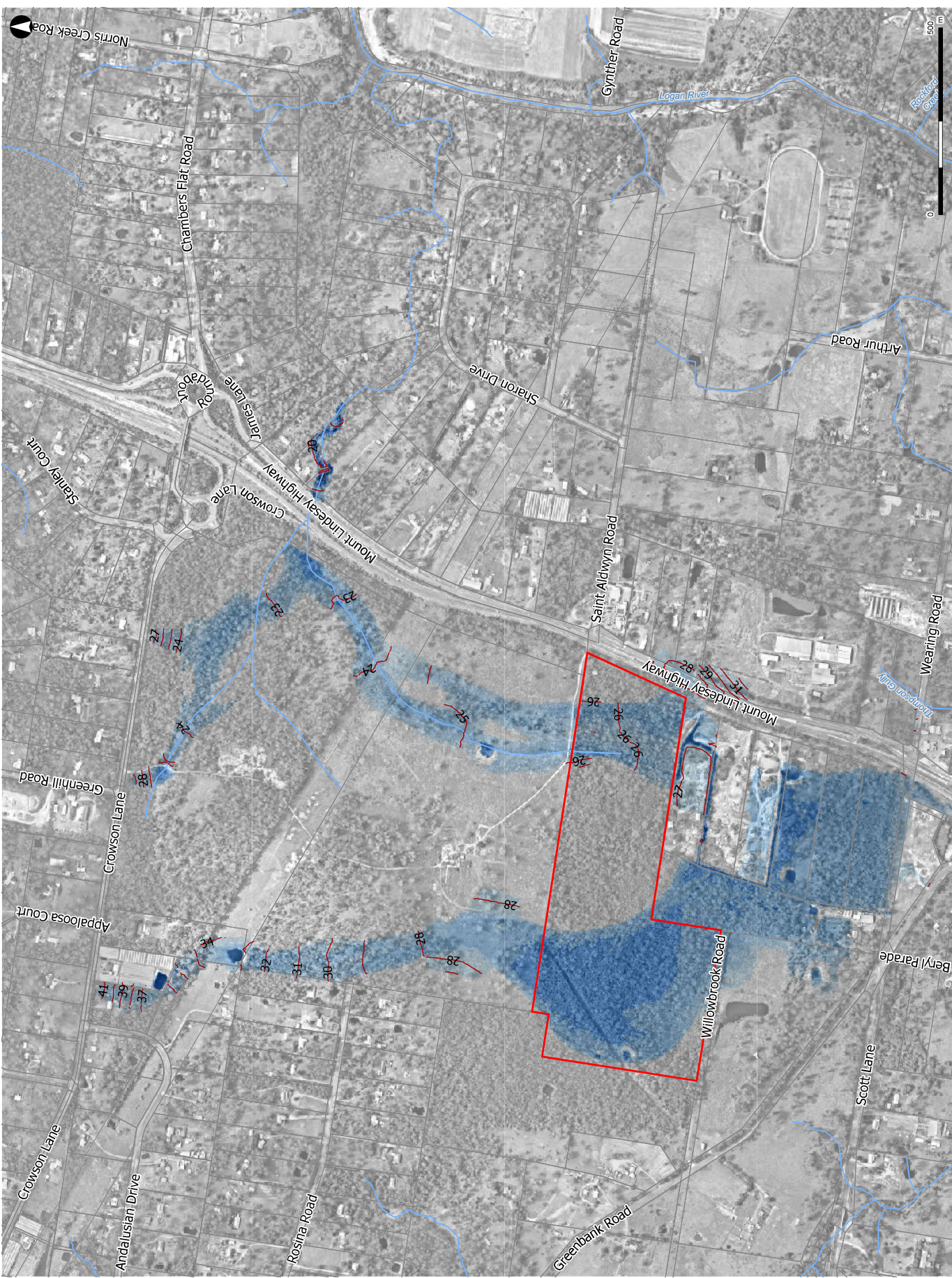
Figure E-5 - Flood Depths - Existing Case 50 year ARI - 2% AEP
