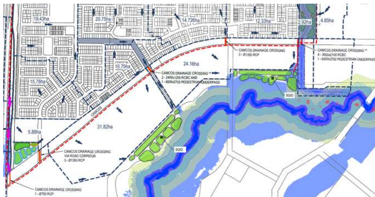
Figure 8: Proposed Drainage Crossing CAMCOS Corridor
