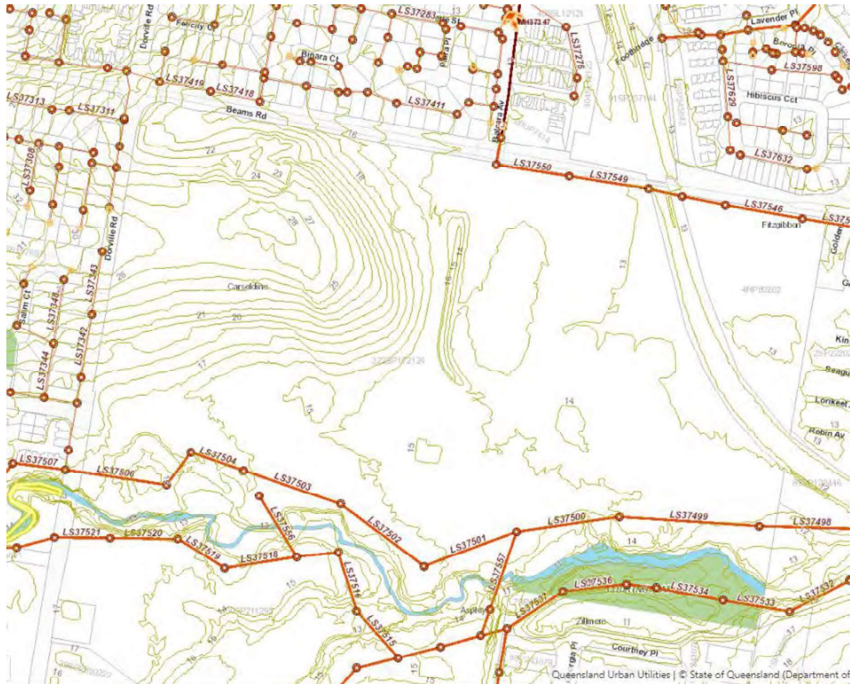
Figure 2 – Development site and surrounding Sewer network
