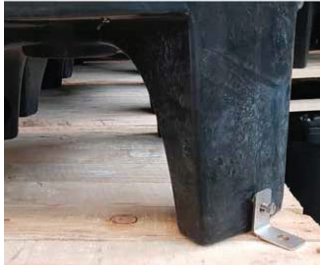
Figure 4 - Bolting the feet
