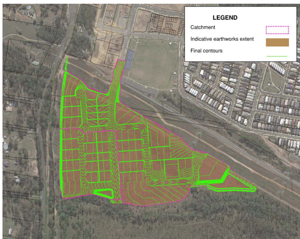
Figure 2: Bulk earthworks extent
