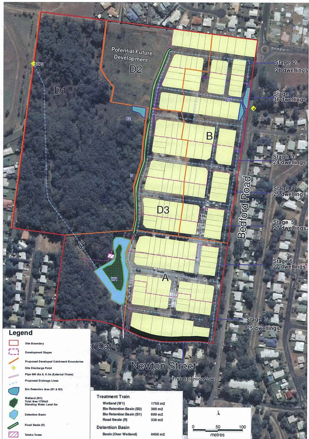
Figure 2.3 Proposed Developed Conditions and Stormwater Management Measures
