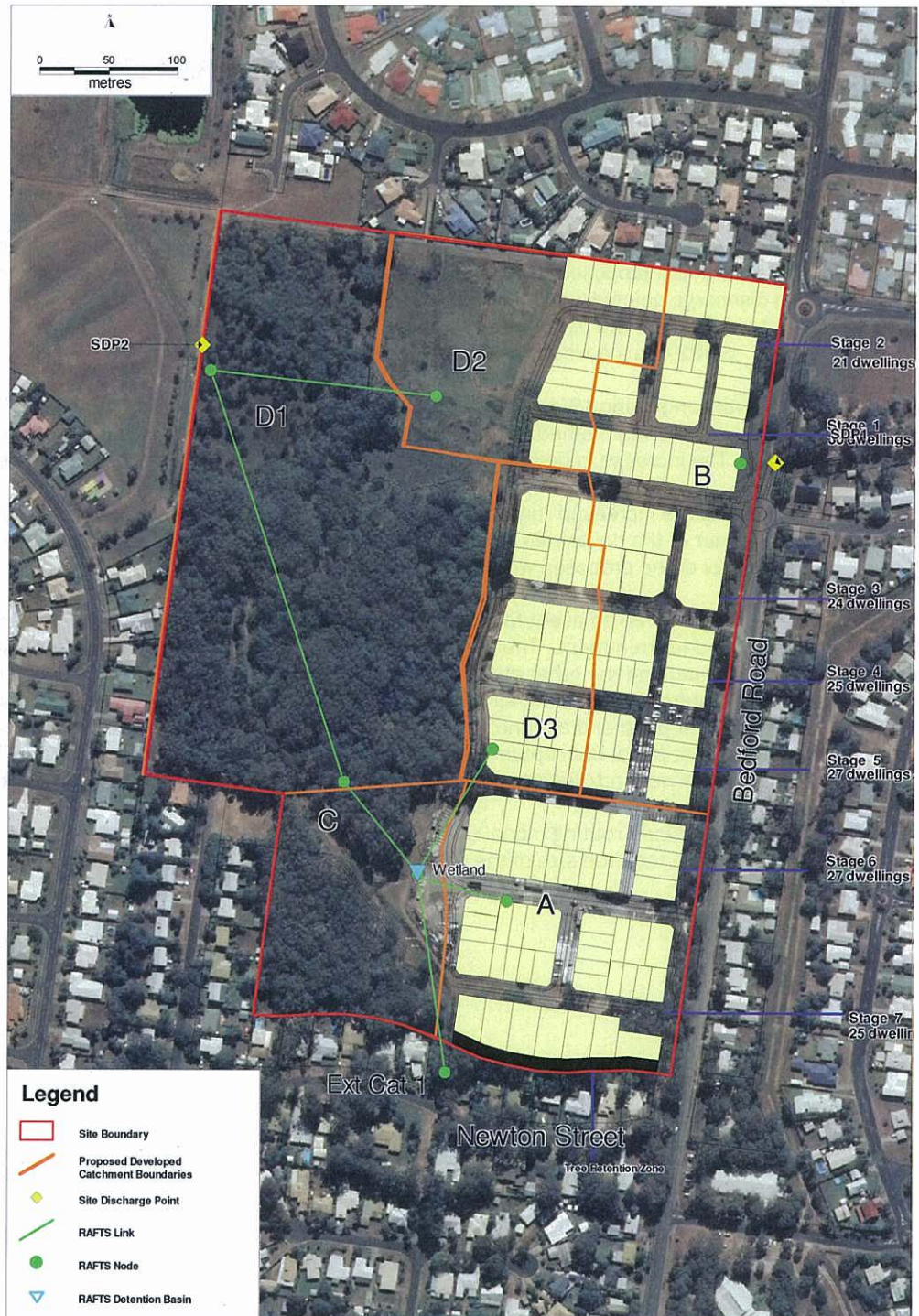
Figure 3.1 Proposed RAFTS Model Configuration
