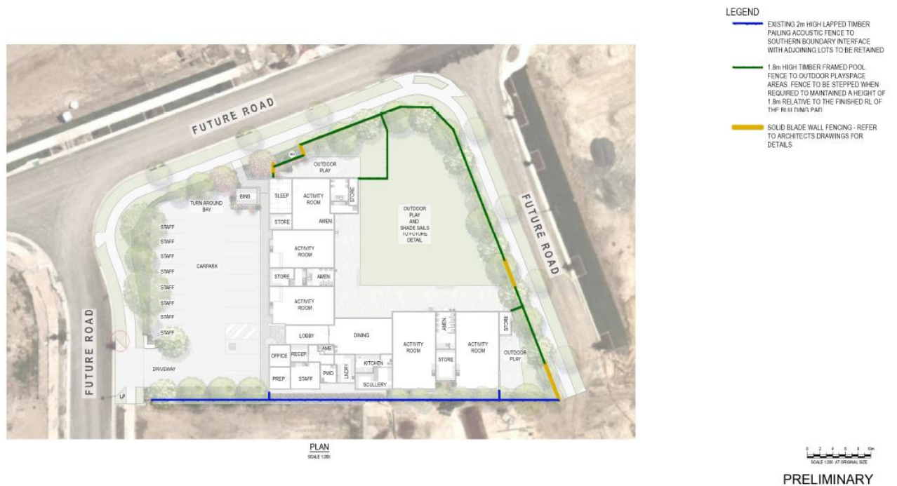
Figure 1: Fencing Plan showing 2 m acoustic fence
