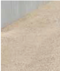
Stabilised Decomposed Granite
