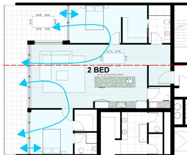
Figure 2: Natural Ventilation – Typical 2 Bed
