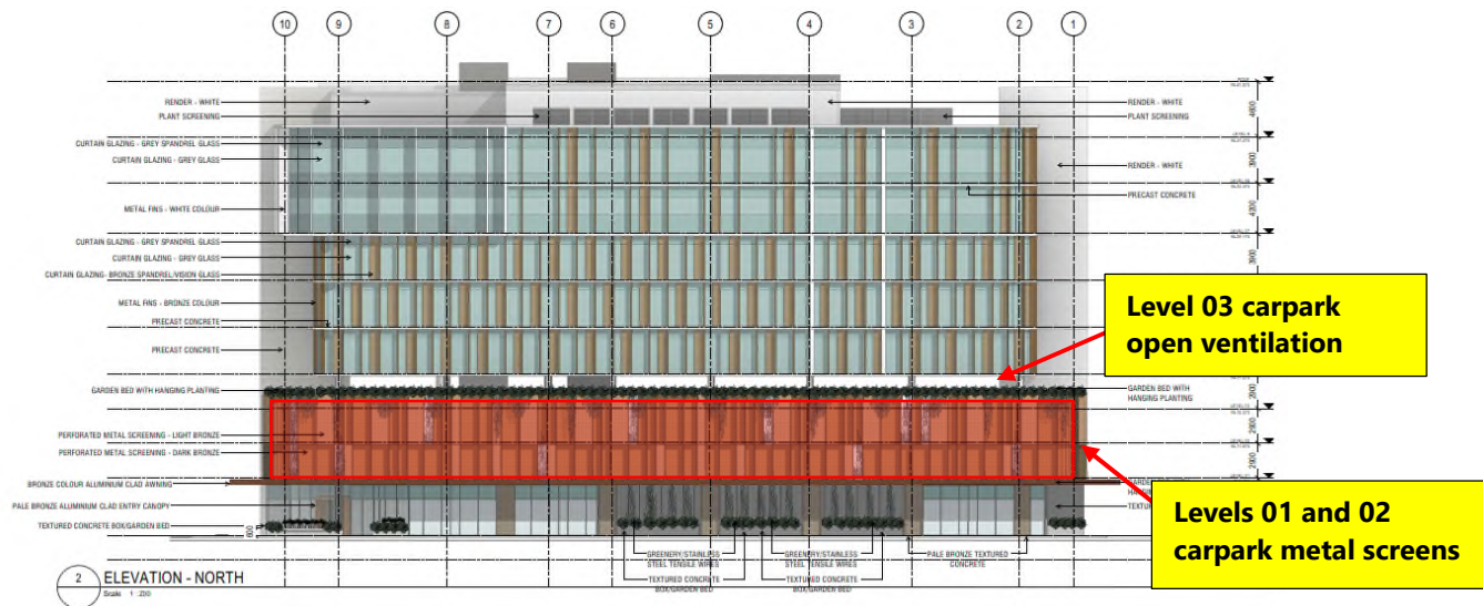
Figure 18: carpark ventilation via metal screens and openings
