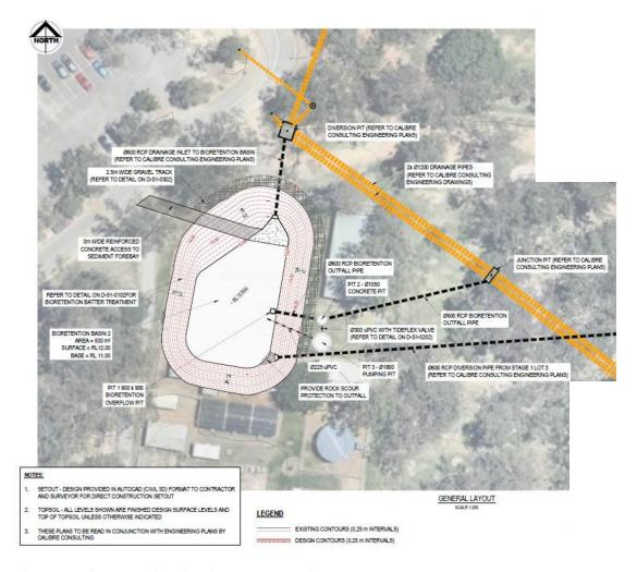
Figure 7 Bioretention basin B2 general arrangement
