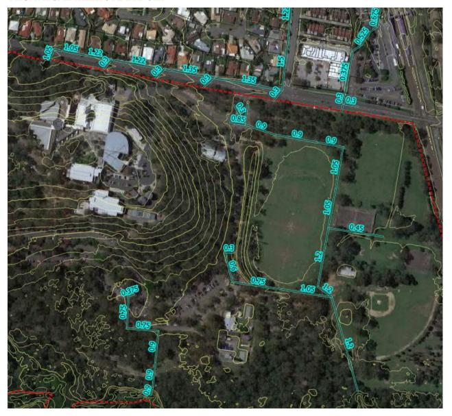
Figure 4 - Existing case pipe drainage and diameters (m)
