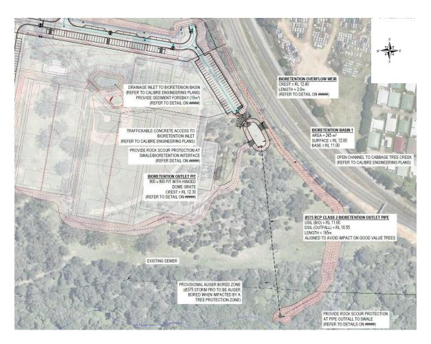
Figure 6 Bioretention basin B1 general arrangement
