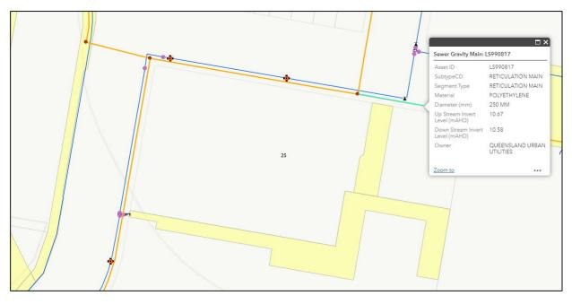
Figure 8.2 Sewer Reticulation Network (Source: Urban Utilities)
