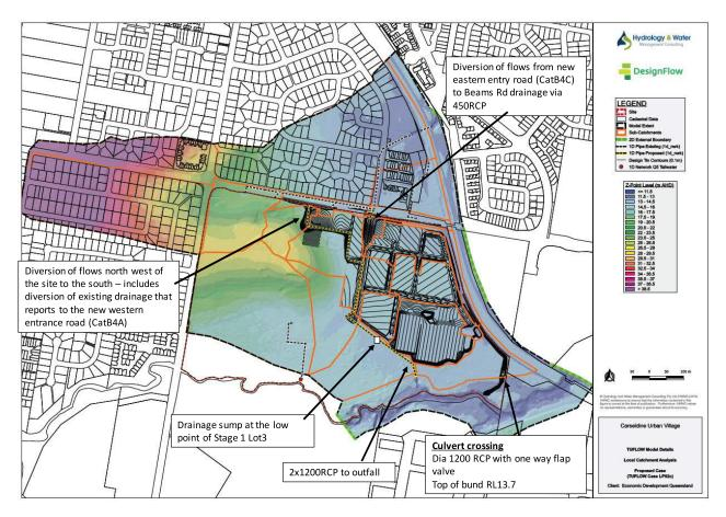
Figure 1 – Local TUFLOW model setup
