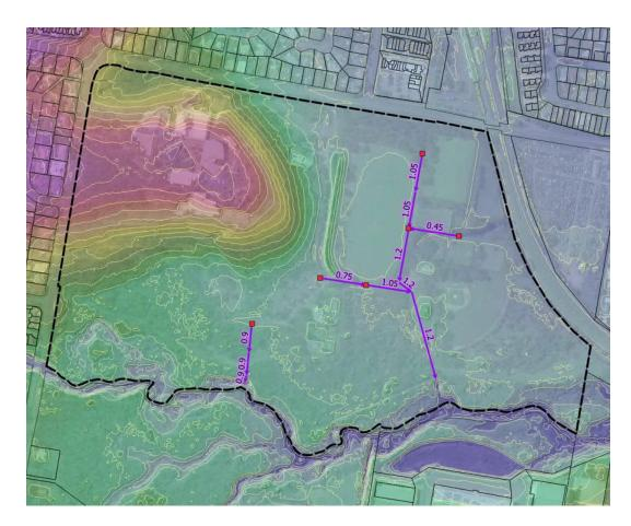
Figure 11 Existing site pipe drainage
