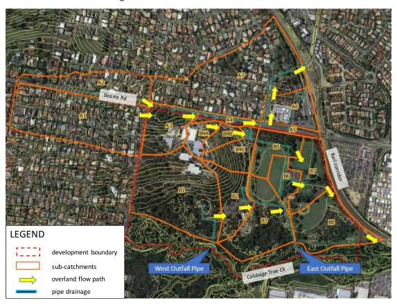
Figure 2 - Existing case WBNM sub-catchments
