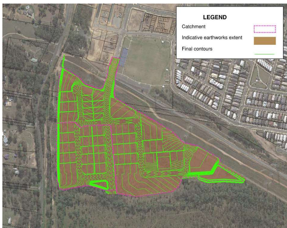
Figure 2: Bulk earthworks extent
