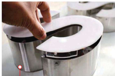
EXAMPLE OF LETTER FACE FIXINGS WITH ACRYLIC TAB
