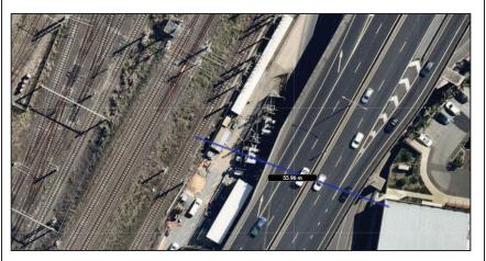
A calculation can also be conducted to estimate the  $L_{Aeq,24hr}$  using the QR tested Sound Exposure Level (SEL) of freight trains. Assuming that freight trains are clearly audible above road traffic and each emit 90 dBA SEL at 25m distance, the estimated number of freight train movements required to meet the 65 dBA  $L_{Aeq,24hr}$  noise limit is 248 trains. This far exceeds the maximum number of 15 freight trains per day reported by QR during the monitoring period. Where
