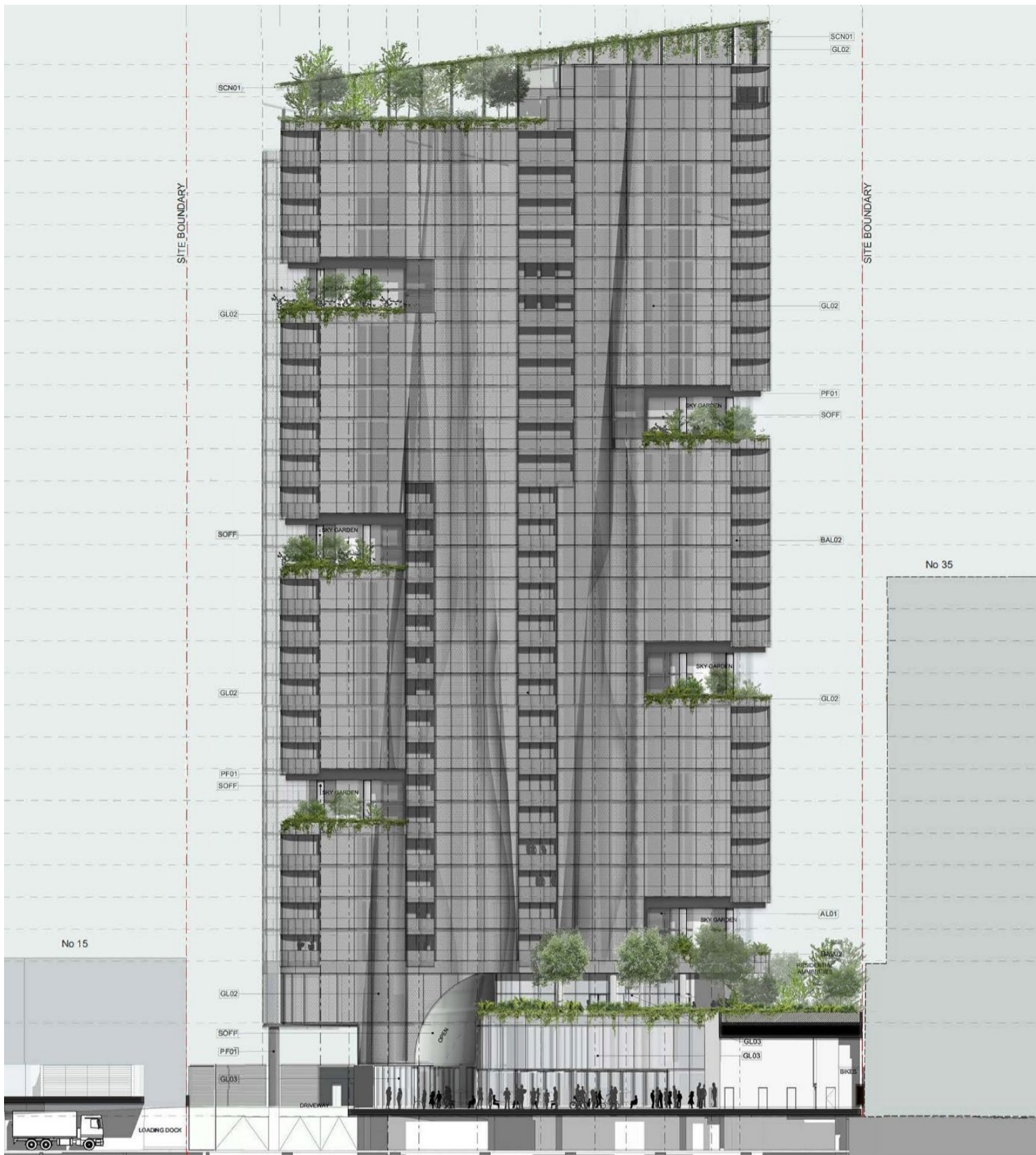
South Elevation – balconies are recessed into the form of the tower.
