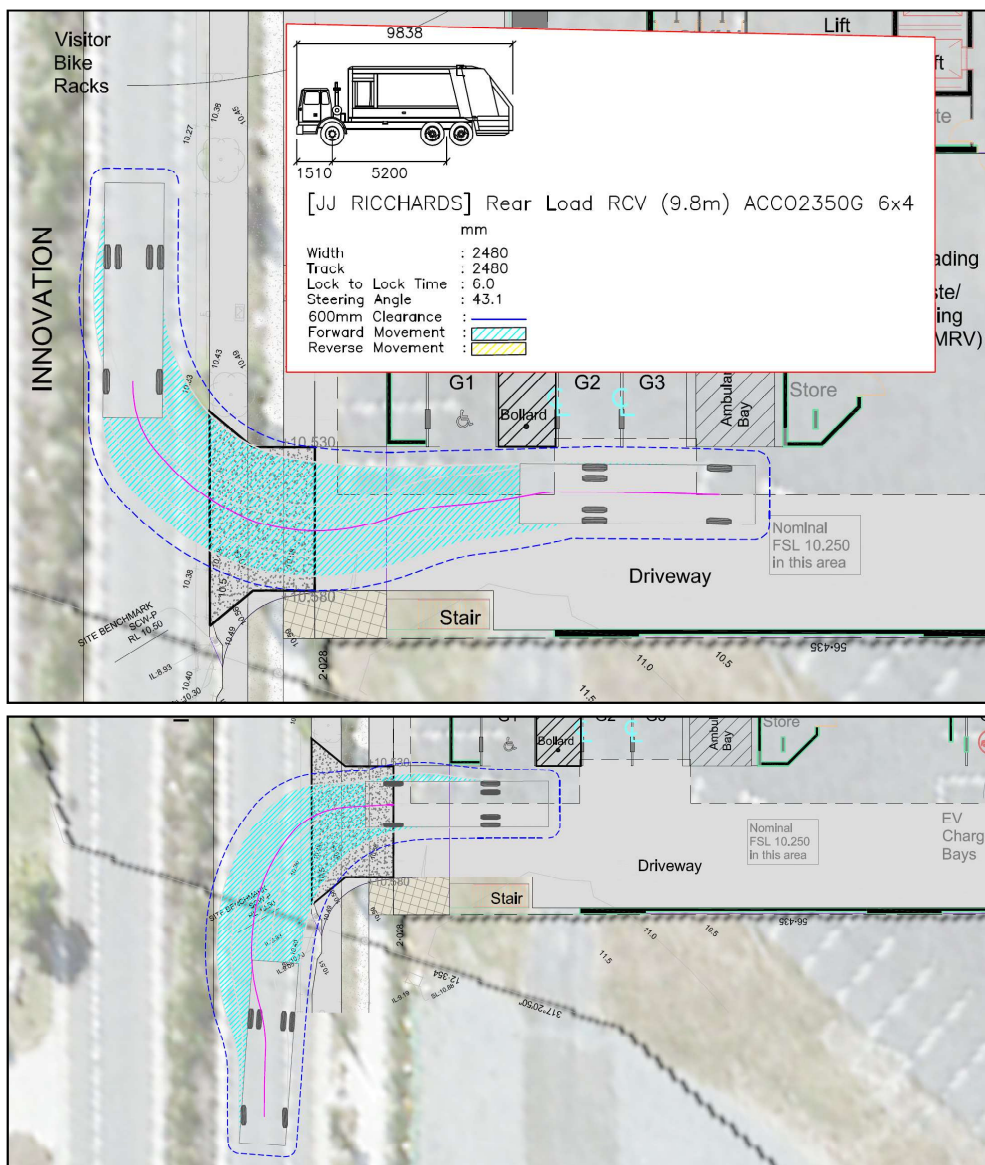
FIGURE 7.1 – REFUSE COLLECTION VEHICLE (RCV) MANOEUVRING (ACCESS)
