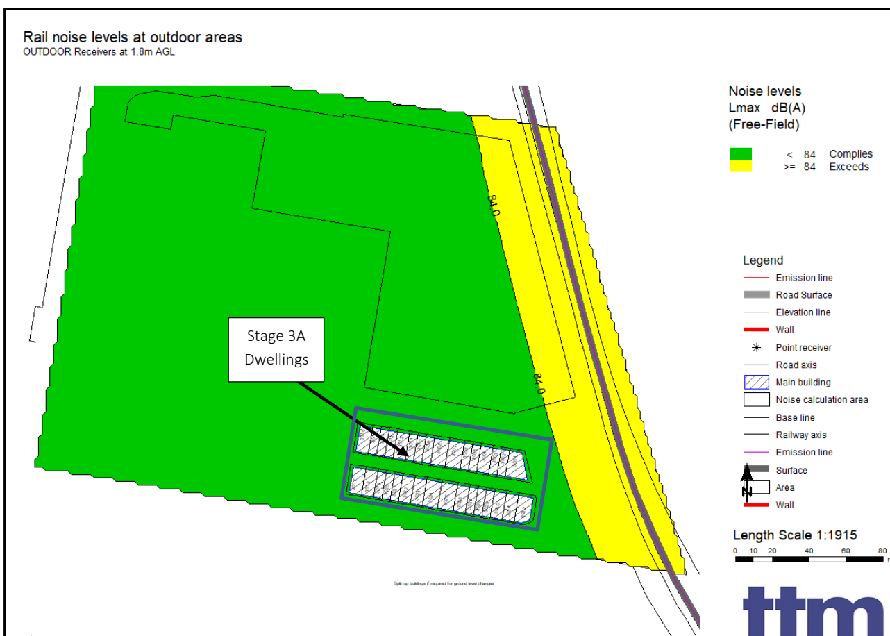
Figure 6: Predicted Rail Noise Levels Compared to SDAP Outdoor Criteria - No Acoustic Barriers
