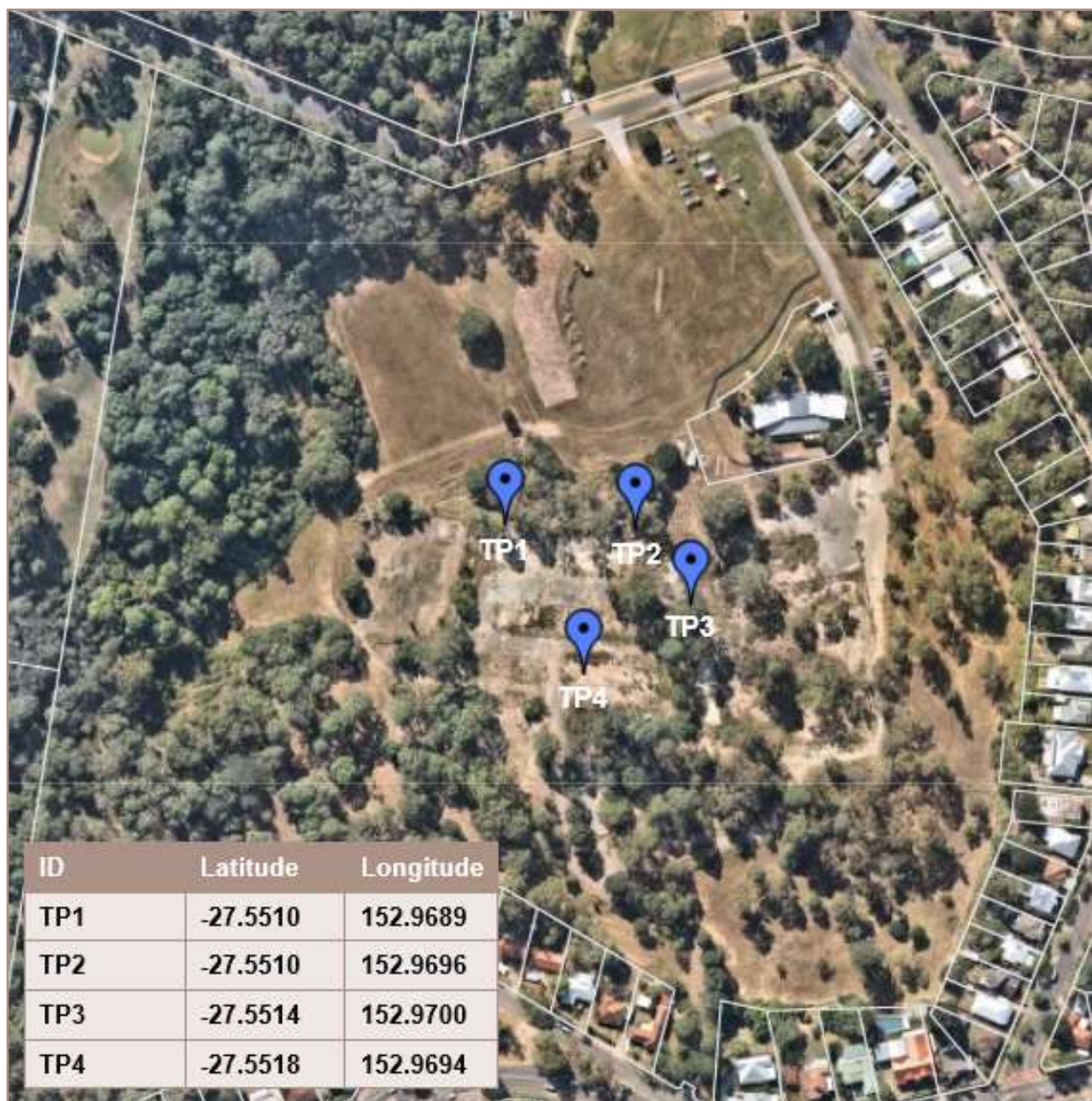
Figure 3-1 Borehole Location Plan
