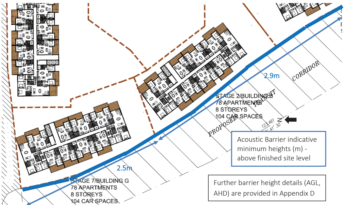
Figure 16: Recommended Acoustic Barrier – Rail Noise - North
