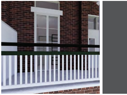
BAL 01 NEW COMPLIANT TIMBER BALUSTRADE & CHARCOAL TOP RAIL TIMBER COLOURS TO MATCH EXISTING
