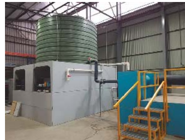
2018, EN 858-1 oil/water separation compliance testing
