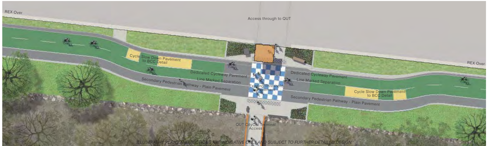
Figure 5.57: Transition Zone E Typical Pavement Treatment
