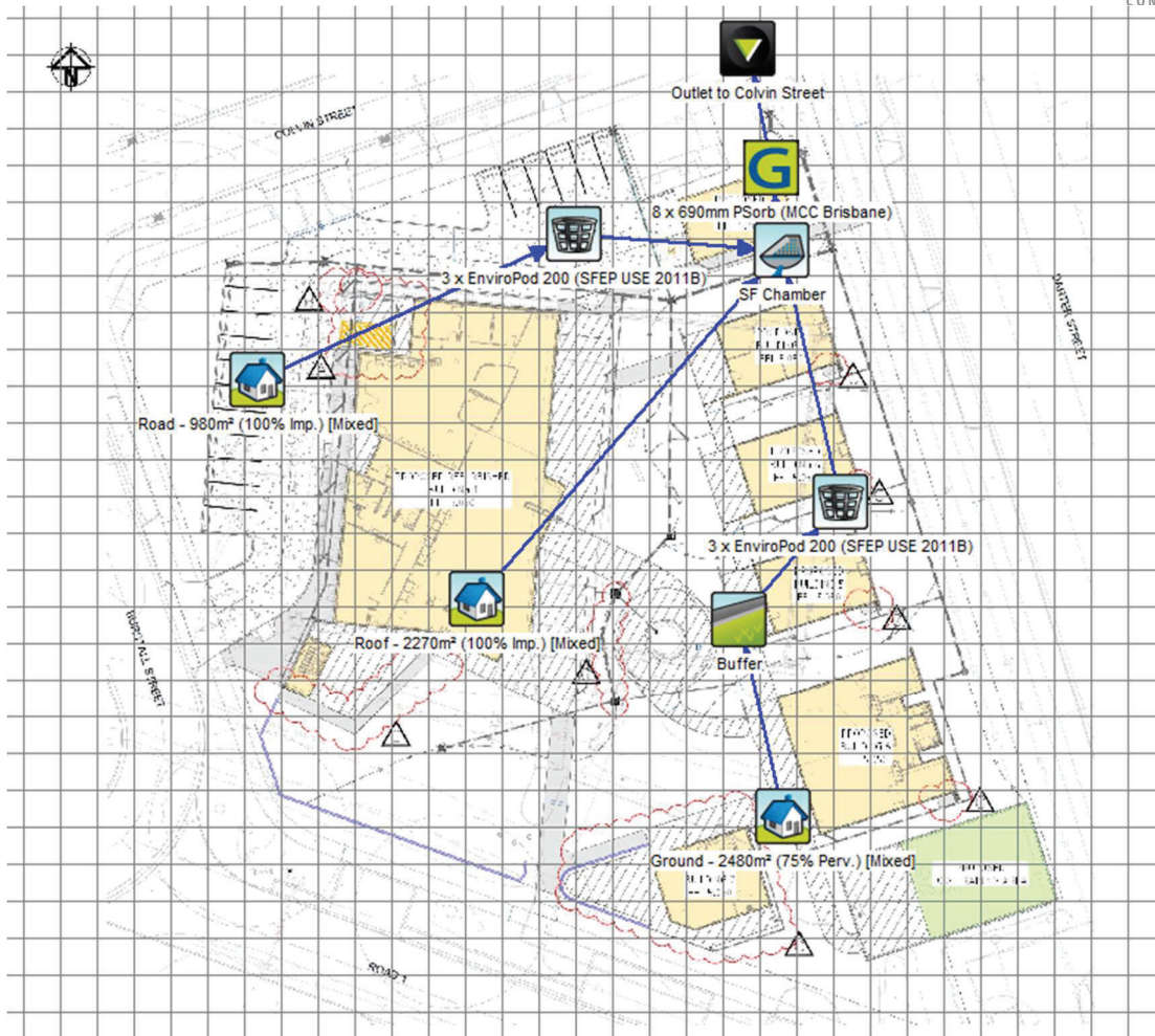
Proposed stormwater treatment train.
