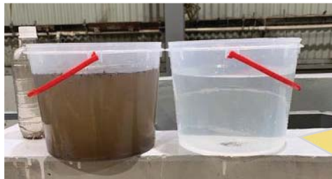
2020, nutrient and fine sediment stress testing, comprises influent dosed with decomposed litter and potting mix
