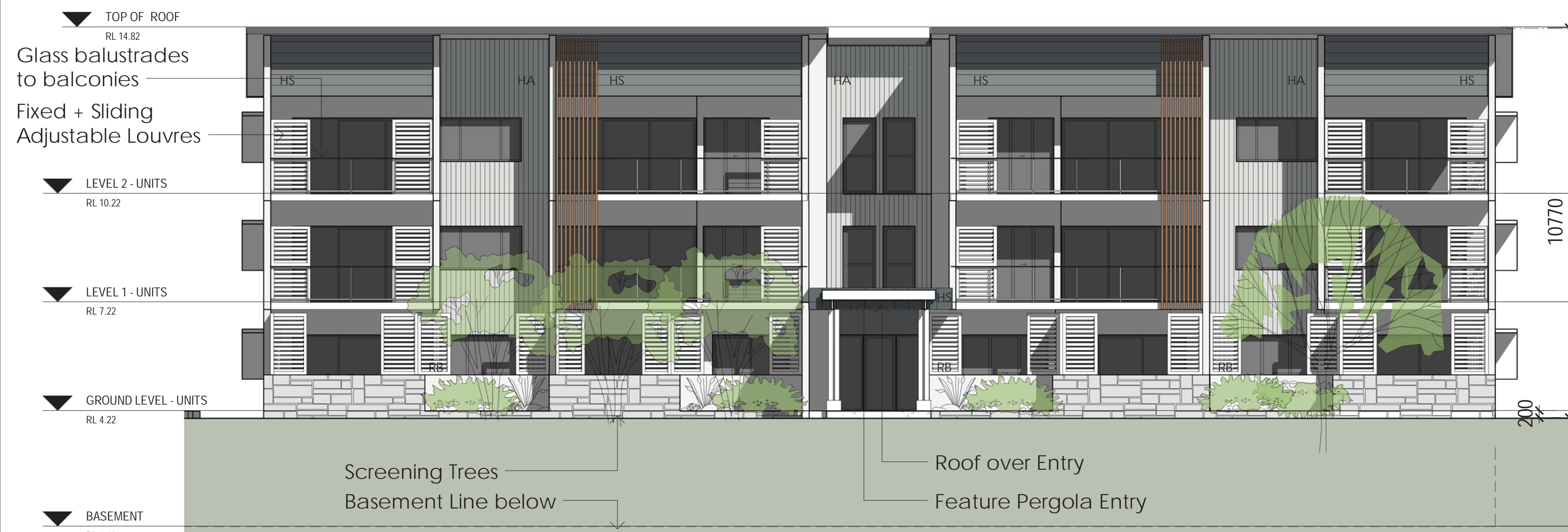
02 South East Elevation - Building 3 1 : 100 @ A1
