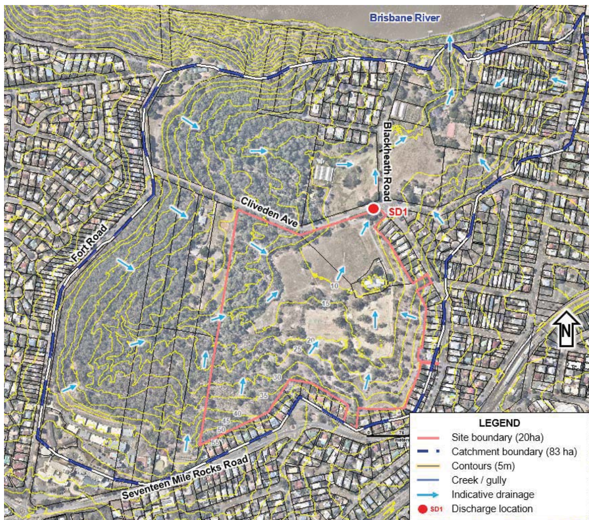
Figure 2: Site Layout and drainage
